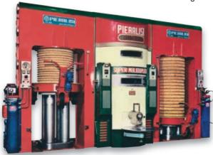
The resulting paste then undergoes a process known as malaxation, during which it is stirred continuously with paddles to encourage the oil to form larger droplets, which makes it easier to separate from the other liquids in the paste. Next, the paste is spread over fibre mats, or filtration diaphragms, which are stacked in a
