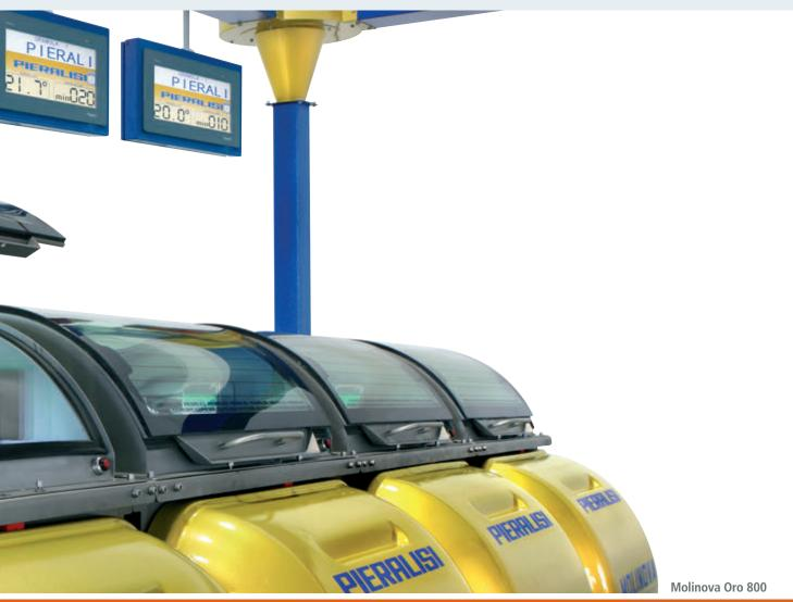
Molinova Oro malaxing system, designed for batch processing, are completely automated and are also able to operate in continuous mode. The malaxer units are made of stainless steel and have a double wall for hot water circulation. Each one has an inspection dome, made of shatter-proof, non-fogging glass, equipped with a safety lock system and a new LED lighting device for easy inside inspection.
