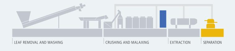
In the last stage of the oil production process, the residual water and solids must be thoroughly separated from the oil coming from the decanter. These residues must also be removed quickly to maintain the high quality of the product.
